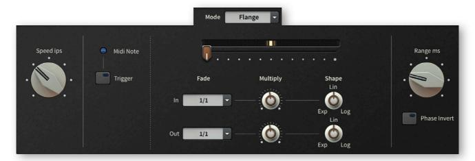
True flanging requires two tape machines running identical recordings. The machines are started at approximately the same position, but while tape1 runs at a constant speed, tape2 is slowed down or sped up manually by applying force on the 'flange' of the supply reel. As tape2 can be running either behind or ahead of tape1, the delay between the two can approach 'zero' from either side: That is what Satin emulates.
